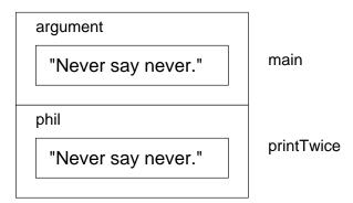
Whenever a function is called, it creates a new **instance** of that function. Each instance of a function contains the parameters and local variables for that function. In the diagram an instance of a function is represented by a box with the name of the function on the outside and the variables and parameters inside.
