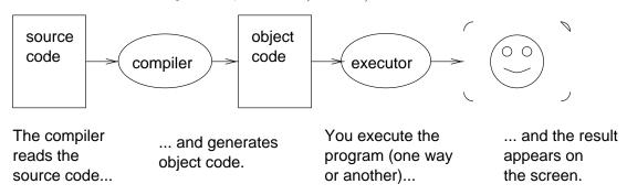
The next step is to run the program, which requires some kind of executor. The role of the executor is to load the program (copy it from disk into memory) and make the computer start executing the program.
