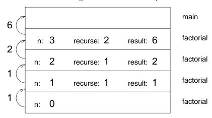
The return values are shown being passed back up the stack.
